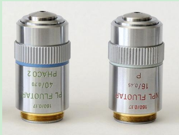
Fig. 6: Leitz objectives used for fluorescence microscopy (PL FLUOTAR 40/0.70 and NPL FLUOTAR 16/0.45).
