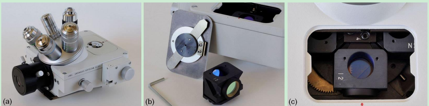
Fig. 3: (a) Leitz Ploemopak 2.2 for Leitz Ortholux II. (b) Leitz filter cube 12 removed from Ploemopak 2.2. (c) Leitz filter cube 12 inside Ploemopak 2.2.
